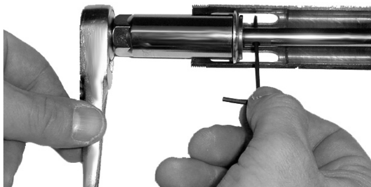
Fig. 1: Removing Grease Intake Assembly
